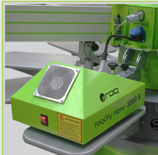
:: LES PRÉ-SÉCHAGES SONT INCORPORÉS DANS LA STRUCTURE DE LA ROQPRINT NANO
