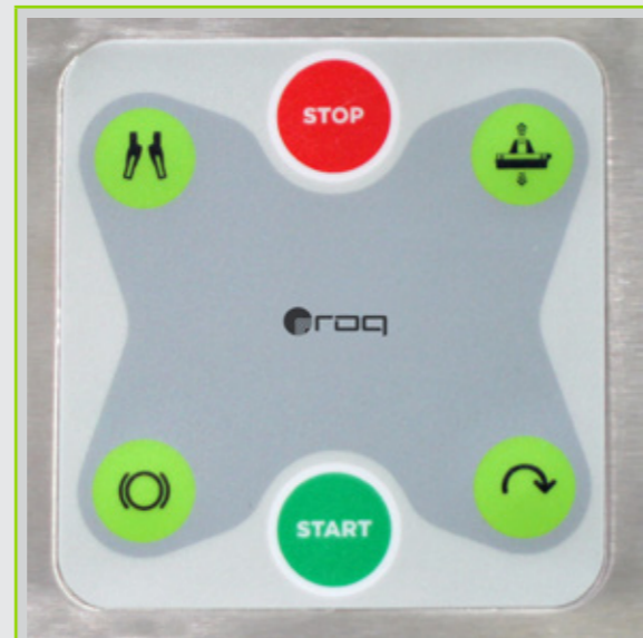
:: COMMAND PANEL IN EACH PRINTING HEAD
