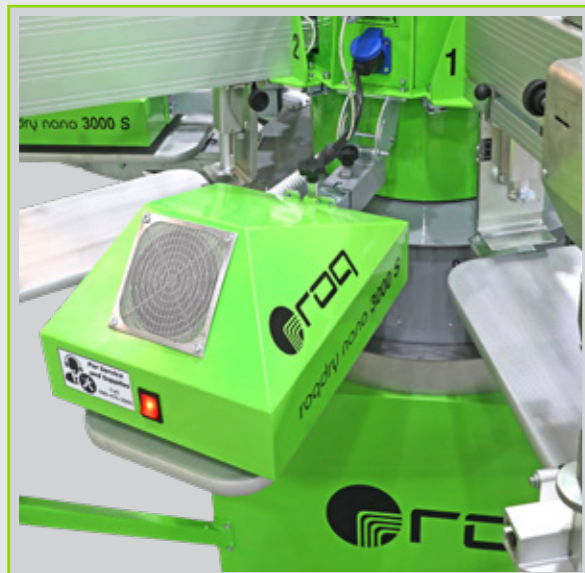
:: NANO FLASH CURE UNIT EMBEDDED IN THE STRUCTURE
